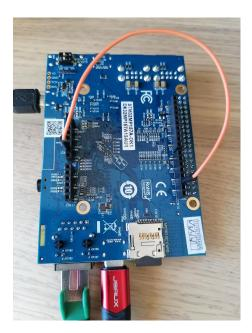
If you check the *Pinout of the Arduino* TM connectors table in the board documentation 8, you will see that the ARD\_D2 pin on the board is connected to the PE1 STM32 pin. PE1 is actually a GPIO pin on GPIO bank E, and is configured as a GPIO by default (no need to change pin muxing to use this pin as a GPIO).
