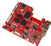
Olimex Open hardware ARM laptop main board
