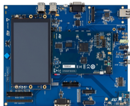
STM32MP157C-EV1 evaluation board
