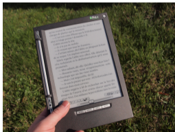
An e-reader with an EPD display
