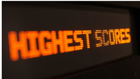
A monochrome dot-matrix display
